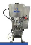
This product is an efficient equipment integrating vacuum mixing and dispersion, which is suitable for the positive and negative electrode slurry mixing process in the battery experiment process. Can be used in various solvents and powder mixing process.
