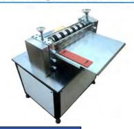
Suitable for slitting of the positive and negative electrode of lithium batteries after coated.
